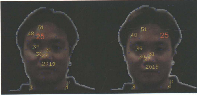
Figure 3-19: The matching of the feature point '25' is regarded to be wrong because the distances between '25' and '35', '48', '51' have great differences in the two images.
